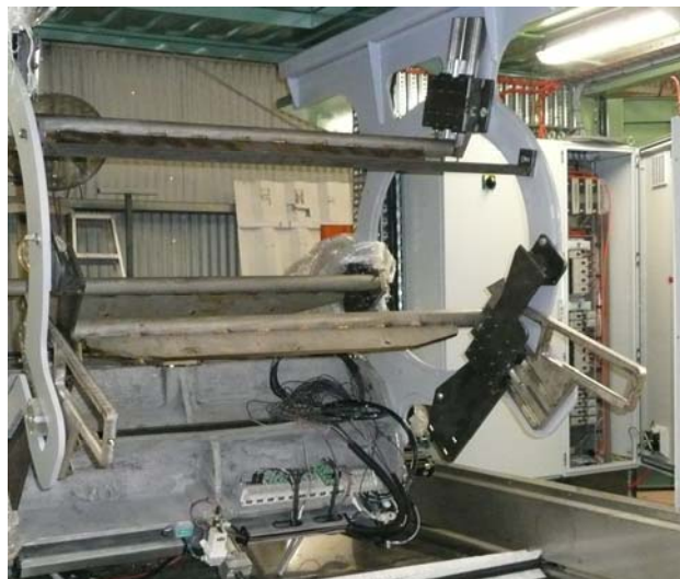
The innovative design of the banana trunk outer layer and inner core conversion processes operating within the modular unit
