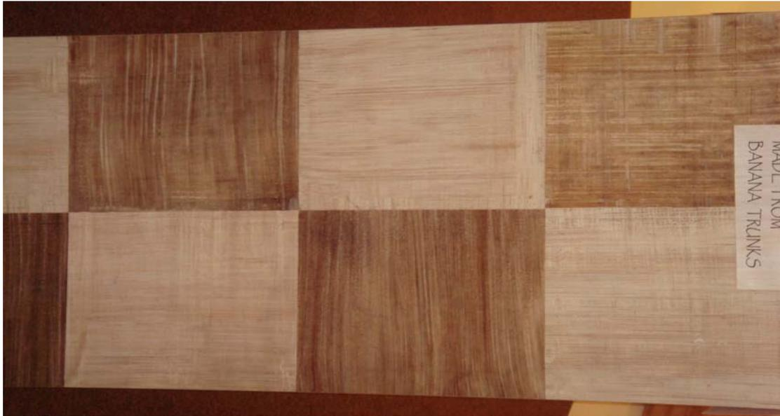
Our banana fibre board product was tested for its fire retardant and water resistant qualities and demonstrated at the exhibition. See the video on the web at [www.papyrusaustralia.com.au](http://www.papyrusaustralia.com.au) or [www.beleaf.tn.mc](http://www.beleaf.tn.mc) which records the fire retardant and water resistant qualities of “Beleaf®” fibre board.
